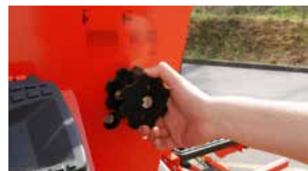
Activating of the half-width shut-off.
