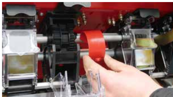
Easy exchange from normal to fine seeds by mounting/dismounting the cover of the crude seed wheel.
