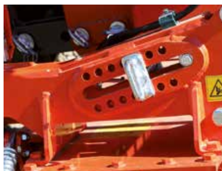
The working depth of the power harrow is easily adjusted on both sides of the machine for a constant harrow and seeding depth.
