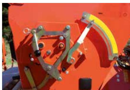
The variable transmission determines the quantity of seed released per hectare.
