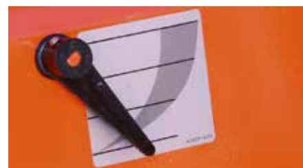
Mechanical level indicator on the seed tank (electronic version available)
