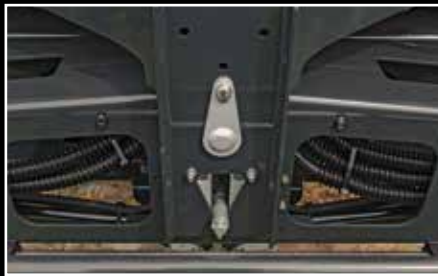
Hydraulic locking pendulum system
