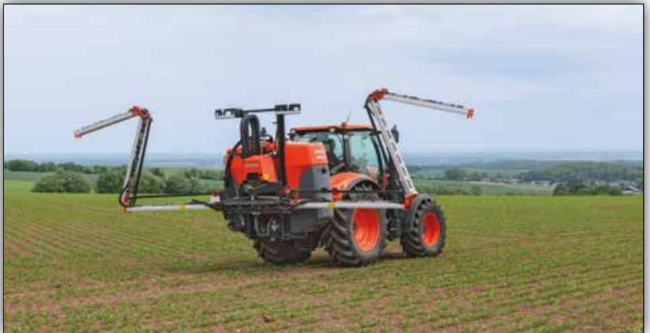
Hydraulic locking pendulum system
