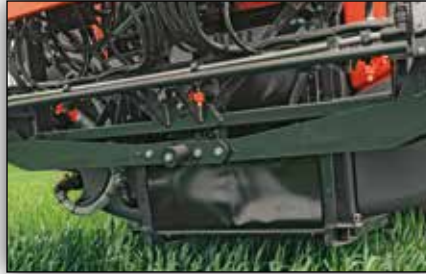
Anti yaw system for independent damping left/right for smooth boom behaviour.
