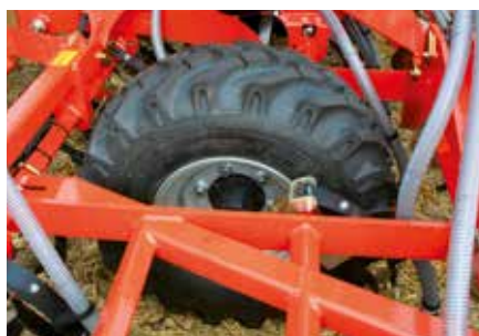
Adjustment of the central wheel by spacer
