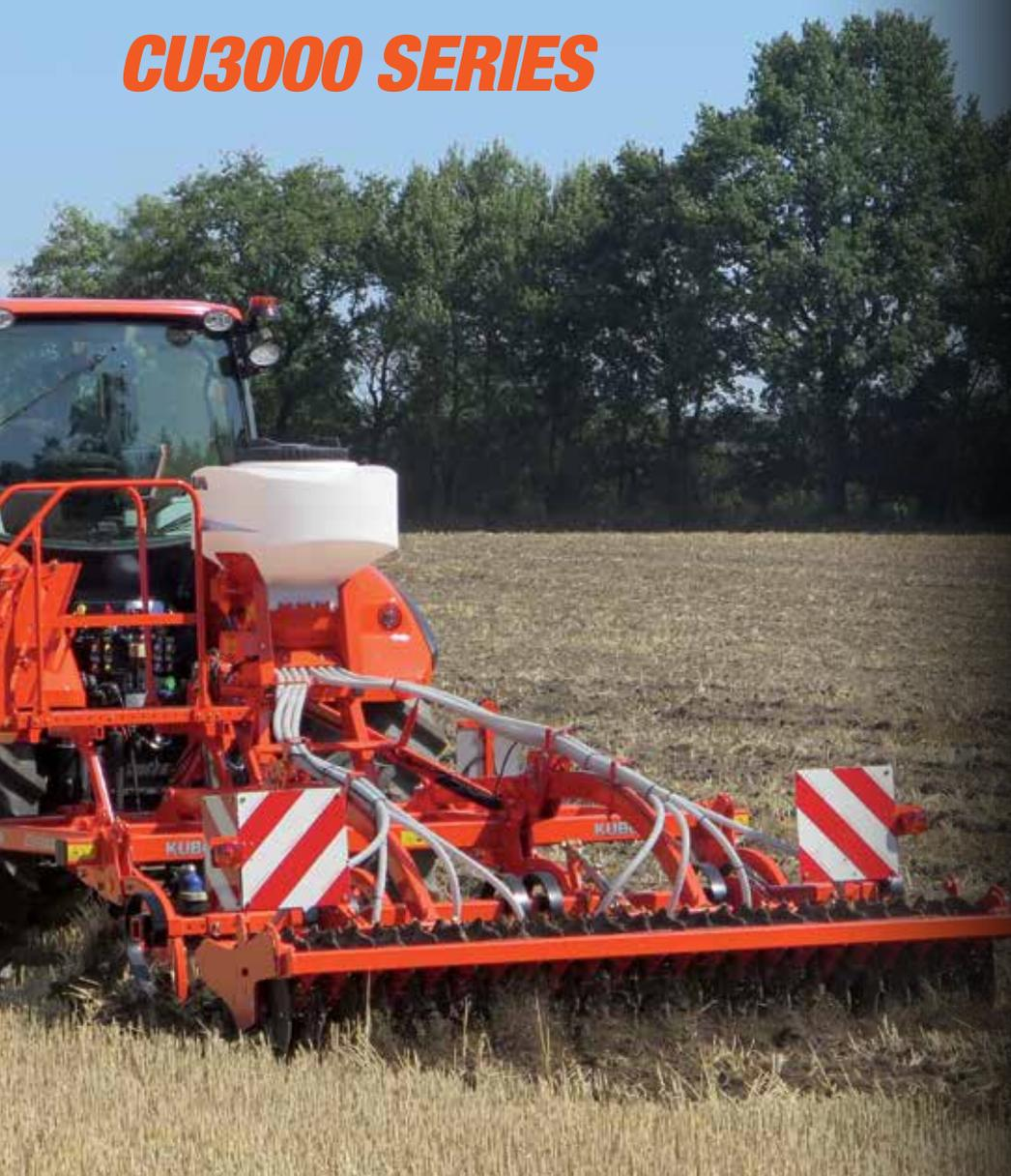
The CU3000 Series has been especially designed to work with the most powerful tractors. With 240HP maximum for 3.00m and up to 350HP for the 5.00m folding model, the Kubota cultivator CU3000 Series has become the benchmark regarding admissible power. It can, therefore, be combined with any type of roller and accessories which makes it extremely versatile. This quality to absorb the strongest forces also ensures a very long durability.
