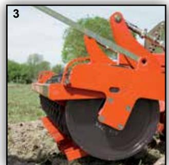
4 different pressures can be applied on the skids depending of the soil nature and the required finish.
